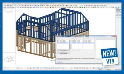
phases or handled by different teams. In such cases, collision control is critical. This will show you immediately and distinguish clearly where components from the D-Ref Building collide with those of the current structure. That way, it is guaranteed that all partial building units are perfectly coming together during construction.
